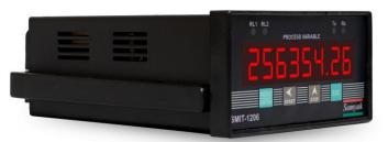
THIS IS A MICROCONTROLLER BASED UNIT. The unit accept various types of field inputs. It displays engineering value of the input & performs integration. The unit can be used as Flow Rate Indicator, Totaliser, Counter or Batching Controller.
