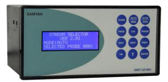
This STREAM SELECTOR UNIT is based on a popular Microcontroller. The system is designed to control the timing of stream selection of up to Four streams system using its timer and relay outputs. It can also generate Sample and Hold type analog outputs for each stream.
