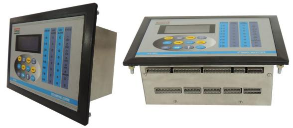
This STREAM SELECTOR UNIT is based on a popular Microcontroller. The system is designed to control the timing of stream selection of up to Six streams system using its timer and relay outputs. It can also generate Sample and Hold type analog outputs for each stream.
